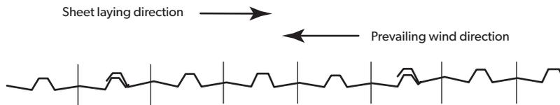
You must lay the first sheet at the opposite side of the prevailing wind direction to ensure lapping is protected from conditions.
