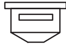
Tapered rainwater heads (downpipe outlet not included) Small: 380 x 175 x 200 mm Large: 450 x 250 x 250 mm Or to your dimensioned drawing.
