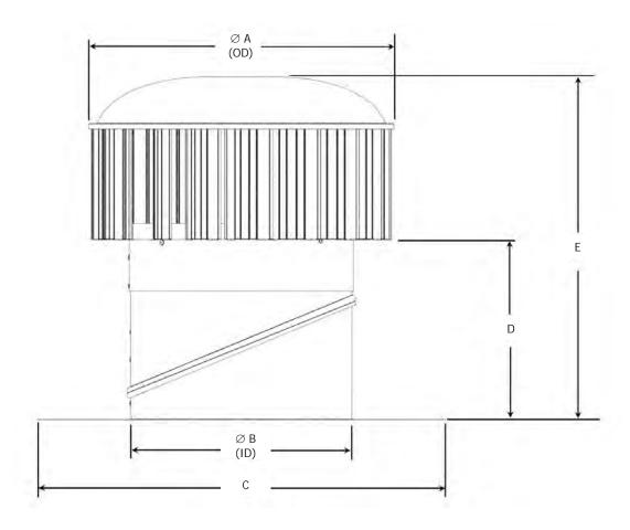
A : Overall turbine diameter B : Internal diameter of flashing opening C: Flashing Overall D : Clearance flashing to turbine E : Overall Height
