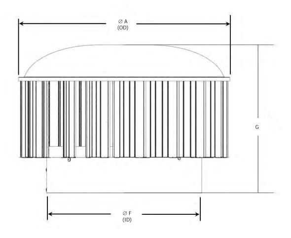
A : Overall turbine diameter F : Effective inner throat opening area
