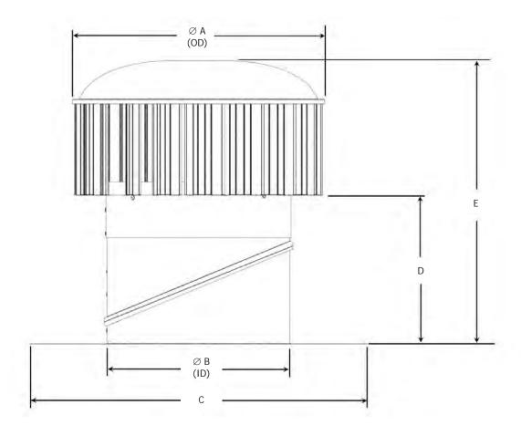
A : Overall turbine diameter B : Internal diameter of flashing opening C: Flashing Overall D : Clearance flashing to turbine E : Overall Height
