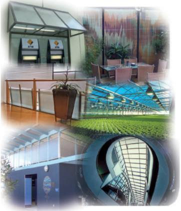
**Lexan\* Thermoclear\*** multiwall sheet is a high quality, low maintenance glazing material that is built to last. Manufactured from Lexan\* polycarbonate resin, it delivers high impact strength, an excellent balance of low weight, and stiffness combined with glass clear transparency.
