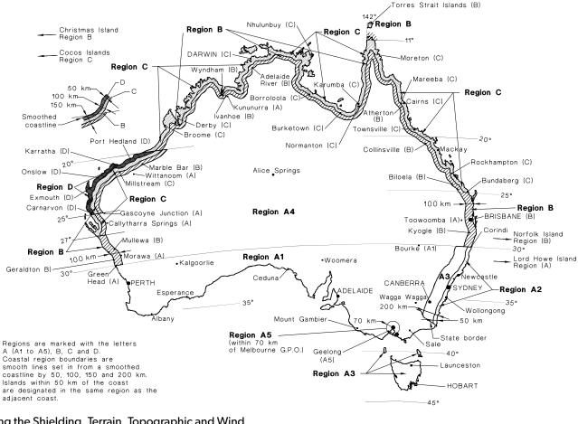
Using the Shielding, Terrain, Topographic and Wind Region data from the information provided here, select your design wind classification from the table below. This allows you to choose the correct Quick Selection table.
