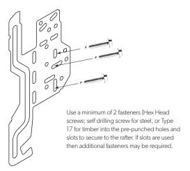
**STEP 2:** Hook the fascia horizontally under each fascia bracket, then flip the fascia forward and lever over the top of the bracket into the vertical position.
