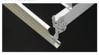
**STEP 3:** Adjust the fascia to the correct position by sliding it along the brackets, then secure the remainder of the intermediate brackets by twisting into fascia first, and then connecting to the rafters.
