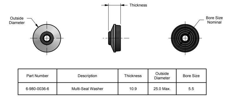
All dimensions nominal unless otherwise stated. Normal manufacturing tolerances apply. All dimensions in millimeters. Third Angle Projection. Scale: Full Size
